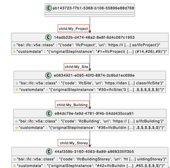
Figure 1: Excerpt from the 'hello-wall.ifcx' example illustrating the USD-style composition model. The project, site, building and storey nodes carry a class label as a string attribute. Their containment relationship is reflected by arbitrarily named child relations.
